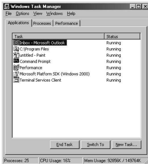
From the Applications tab, you can match a task to the process that owns the thread that owns the task window by right-clicking on the task name and choosing Go To Process.
