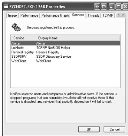
The information displayed includes the service name, display name, and service description, if it has one, which Process Explorer shows beneath the service list when you select a service.
