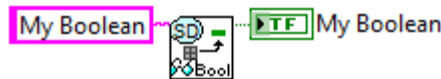
FIGURE 8.3 Reading a Boolean value stored in the network table. Note the cute reading glasses to indicate that we are reading data.
